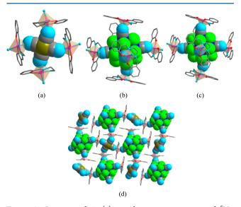
**Figure 2.** Structure of 4: (a) coordination environment of [Ni-(CN)<sub>4</sub>]<sup>2-</sup>; (b) trans-coordination environment of the [Nb<sub>6</sub>Cl<sub>12</sub>(CN)<sub>6</sub>]<sup>4-</sup> unit; (c) cis-coordination environment of the [Nb<sub>6</sub>Cl<sub>12</sub>(CN)<sub>6</sub>]<sup>4-</sup> unit; (d) projection of the overall structure showing the disorder of the [Ni(CN)<sub>4</sub>]<sup>2-</sup> unit.
