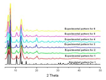
**Figure 3.** Comparison of the experimental powder XRD patterns of the six compounds at room temperature against the simulated pattern from a single crystal of 1. The simulated powder XRD patterns of 1, 2, and 4–6 are similar, so only that of 1 is shown here.
