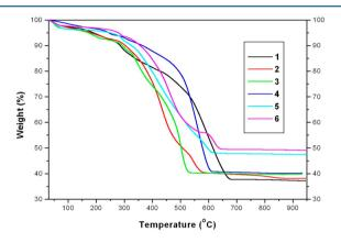
**Figure 5.** TGA plots for the six compounds heated from 30 to 950 °C at 5 °C/min in air (40 mL/min).
