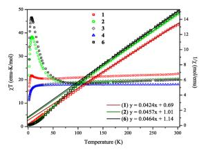
**Figure 6.** Magnetic susceptibility  $(\chi T)$  plotted versus temperature (K) between 2 and 300 K for compounds 1, 2–4, and 6. Reciprocal magnetic susceptibility  $(\chi^{-1})$  for compounds 1, 2, and 6, with their respective equations for the Curie–Weiss law.
